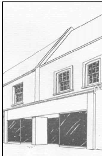
Left: Lack of stall risers at ground floor level resulting in an unbalanced shop front
