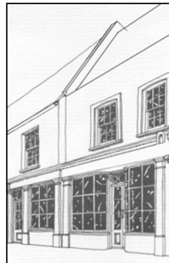
Right: Same shop front but with stall risers, dividing pilasters and cornices
