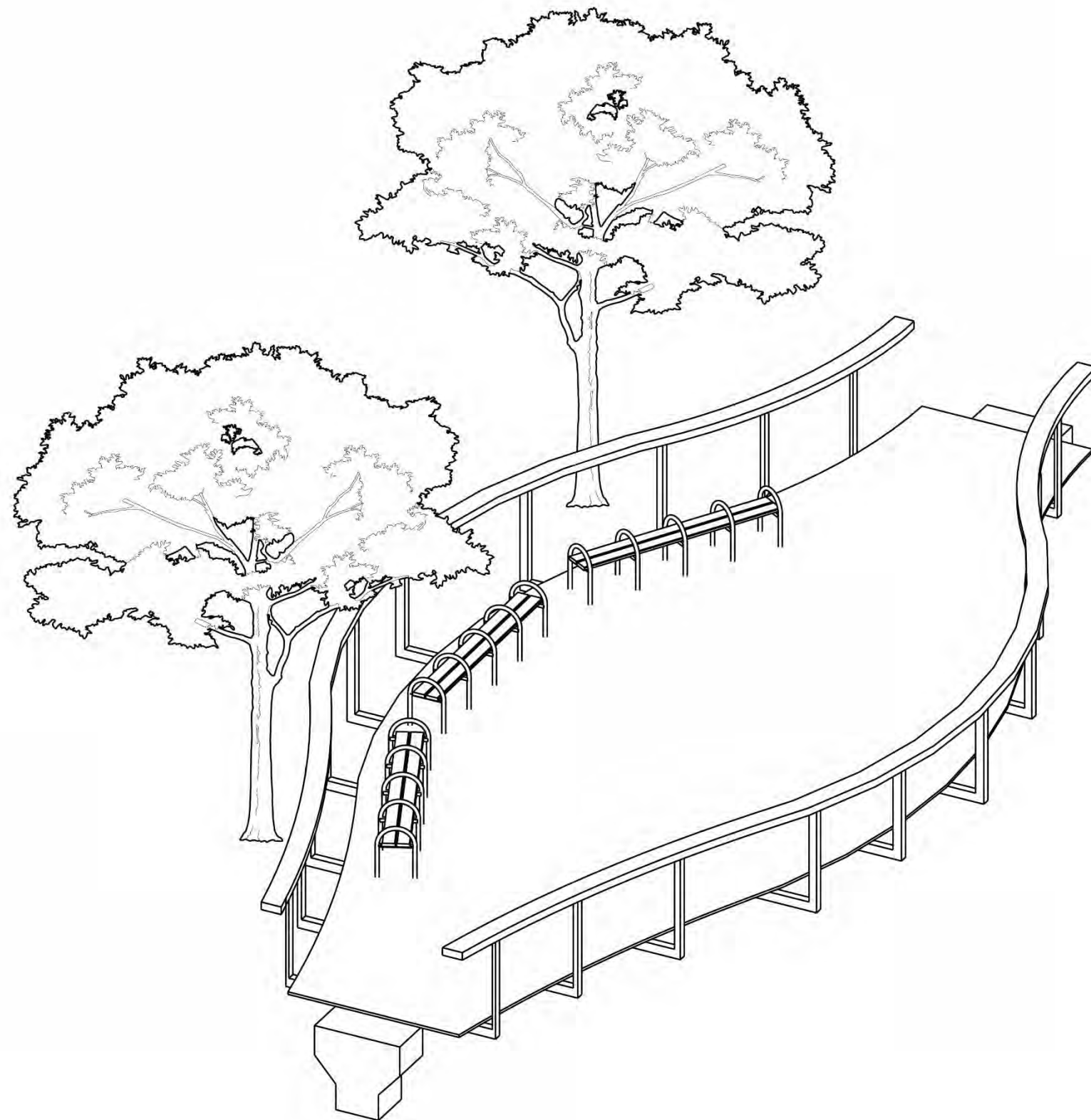
Figure 7A.16.11 Image showing how wider and narrower sections could allow passing. This could also include seating. (Not to scale).
