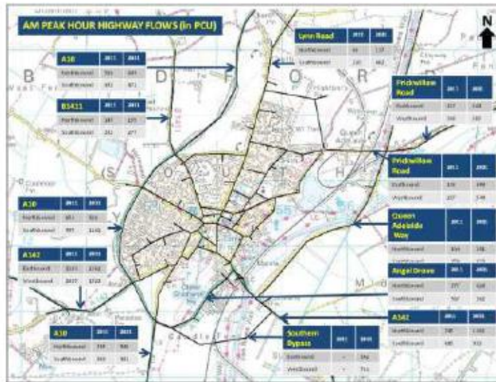
©Crown Copyright 2012- Cambridgeshire County Council OS Licence Number 100023205 Figure 4: Changes in highway link flows in the morning peak between 2011 and 2031. Source : East Cambridgeshire Local Plan Transport Test (October 2012).
